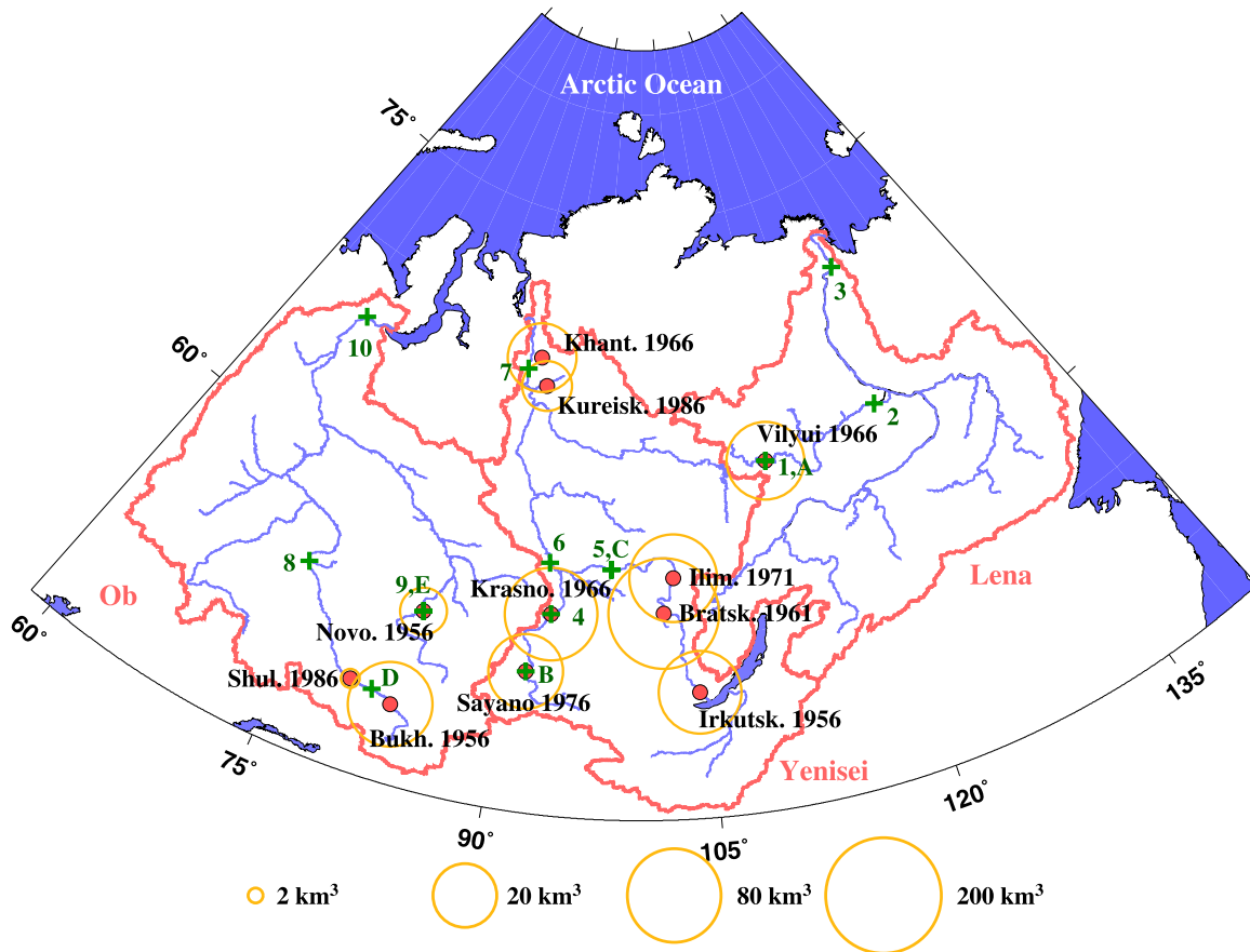
Figure 1. Locations of operational reservoirs for which the storage capacities exceed 1 \text{ km}^3 (shown as solid red circles) for the Lena, Yenisei, and Ob' river basins (see Table 1 for reservoir characteristics). The storage capacities of the reservoirs are given on a log ten scale by the diameters of the yellow circles. The green pluses indicate the locations of the streamflow gauging stations used either for bias correction of inflow into the farthest upstream reservoir on each tributary (letters A–E, see Table 2 for station information) or for reservoir model evaluation (numerals 1–10, see Table 5 for station information). Some stations are used for both purposes. If a green plus is located directly over a reservoir station, this indicates that the gauging station is just downstream of the reservoir outlet. Note that Boguchanskoe reservoir on the Angara tributary (located at gauging station 5) is not shown because it is not yet operational.
